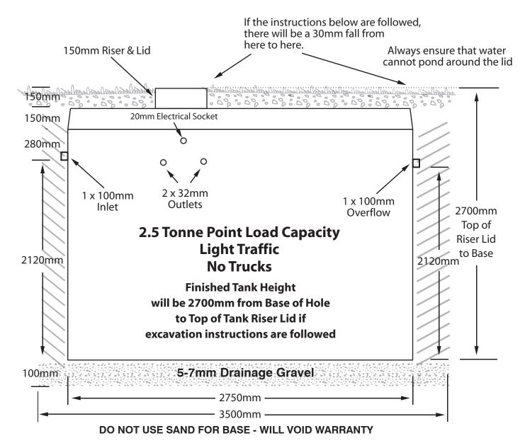
Tanks must be installed perfectly level. Failure to do so will void warranty.
