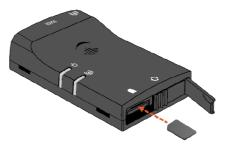
**To close**, slide the cover back to the left, and then push the right side flap closed.
